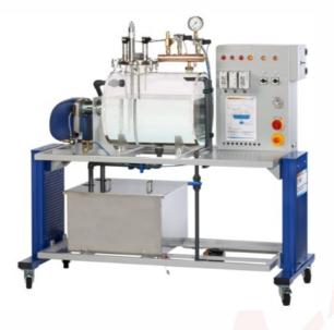
**Introduction:** The Pressure And Temperature In A Steam Boiler Are Increased By Constantly Supplying Energy So That The Liquid Medium (in Most Cases Water) Becomes Gaseous. Steam Boilers Are Monitored By Safety Devices Which Are Electrically Connected In Series, The So-Called "safety Chain". If One Of The Monitoring Or Control Devices Trips, An Alarm Is Triggered And The Entire System Or The Affected System Component Is Switched Off.
