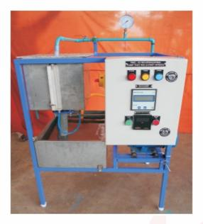
In general a pump may be defined as a mechanical device which when interposed in a pipeline, converts the mechanical energy supplied to it from some external source into hydraulic energy and transfers the same to the liquid through the pipeline, thereby increasing the energy of the flowing liquid. The various pumps may broadly be classified into the following two types:
