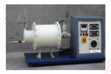
The apparatus consists of a metal bar whose one end is heated by an electric heater & the other end is kept in a cooling water chamber, which acts as heat sink. The test section, i.e. middle portion of bar is provided with thermocouples. Test section is well insulated to minimise radial heat loss.
