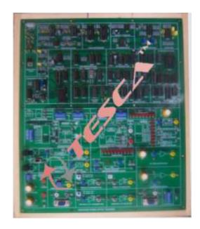
**Order Code- 28527** is a single board Fiber Optic Trainer Kit to study the characteristics of Fiber using Digital and Analog techniques. This kit also facilitates with digital and analog Modulation & Demodulation communication techniques.
