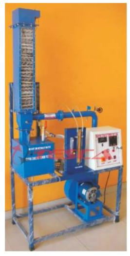
The apparatus consists of a forced draught, counter flow type-cooling tower. A blower supplies cooling air. Air enters the tower at the bottom. Hot water is, obtained from a geyser. Hot water is sprayed over the mesh packing through the nozzles and it flows downwards. Evaporative cooling of water occurs due to the current of air and water gets cooled. This student can study the operation of cooling tower and Calculate the energy balance.
