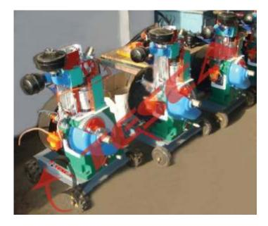
4 Stroke 1 Cylinder Diesel Engine - Manual Driven
