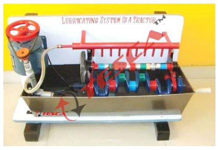
Lubrication System of an Automobile
