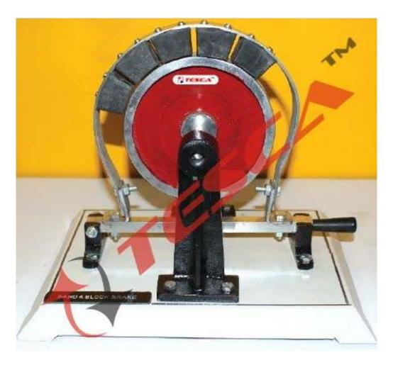
Band & Block Brake - Working Model
