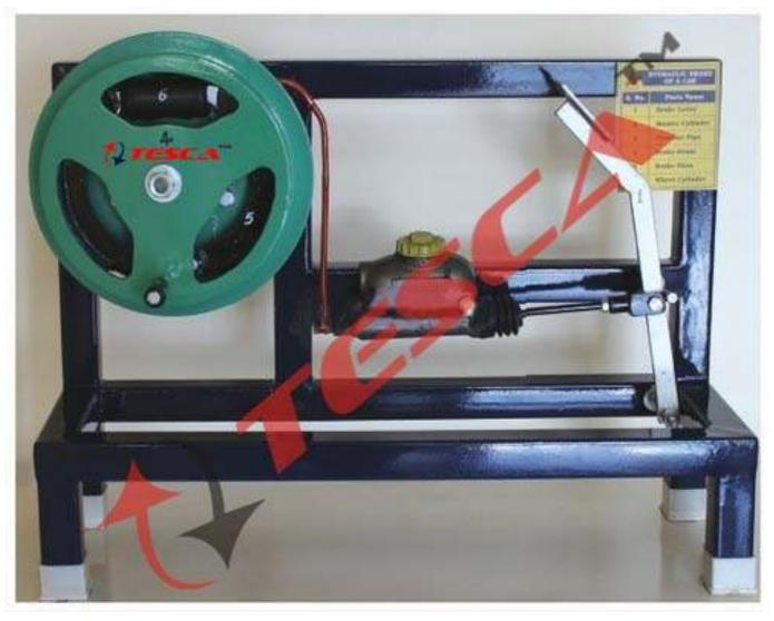
Hydraulic Drum Brake Actual Working (Single Drum)
