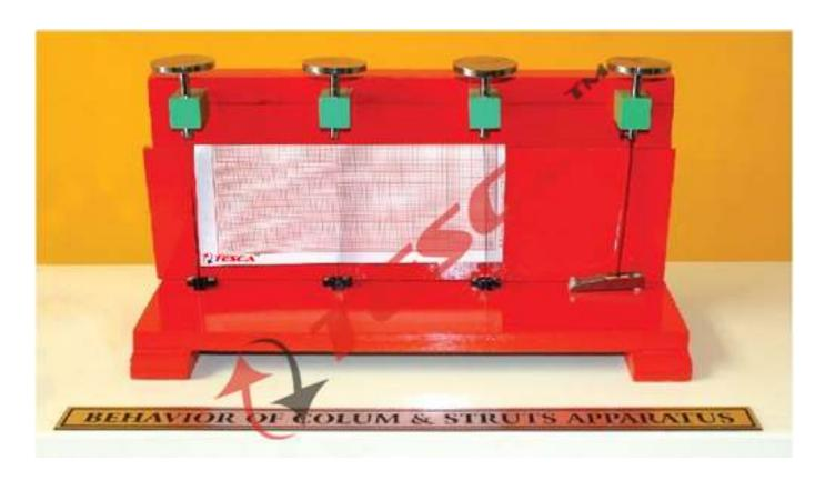
Apparatus consist of four spring steel columns which are put along a vertical wooden board. These four columns have different end conditions as below:
