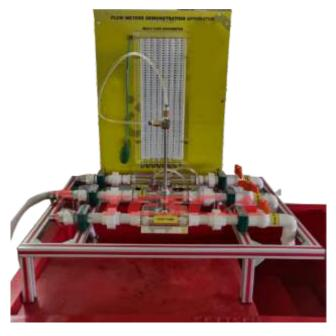
orifice meter, rotameter etc. The flowmeter to be calibrated can be fitted to the apparatus. The apparatus will have a master flow sensor with accuracy of +/- 2% which can be used as a reference for calibration of flowmeter.
