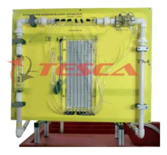
Various devices are available to measure the fluid flow rate. Majority of these devices use Bernoulli's theorem which states that the sum of pressure head, velocity head and the potential head is constant along a streamline for a steady, inviscid and incompressible flow of fluid. Measurement of fluid flow rate is important to the students of mechanical, chemical, civil and several other branches of engineering.
