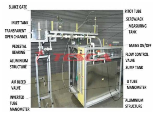
Study of open channel flows and visualization of flow patterns around objects is a subject of interest in basic fluid mechanics. A small flow channel with a provision to control flow velocity and to inject dye into the flow can provide a very useful tool to study several aspects of potential flow and streamline patterns. Flow visualization channel is an important apparatus for students in fluid mechanics, hydraulics, civil, mechanical and related areas in science and technology.
