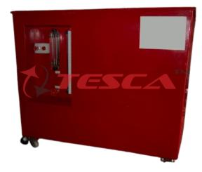
Tesca Basic Hydraulic Bench is of volumetric type and has been designed to provide a continuous and controlled supply of water to conduct various experiments using auxiliary modules in typical Fluid Mechanics and Hydraulics Laboratory. The unit is an ideal service unit for conducting student projects. Once filled, no external water supply is required. Water is recycled between the Experiment Module, Measuring Tank, and the Storage Tank by the Centrifugal Pump.
