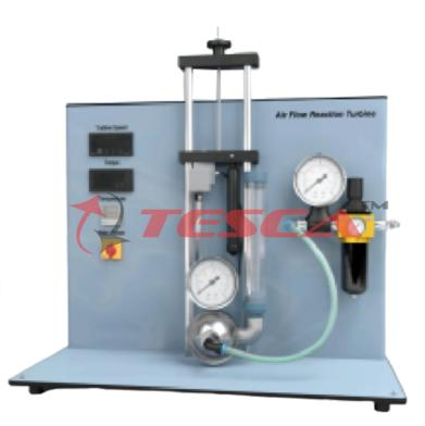
for applying a load to the turbine. The number of active nozzles can be adjusted by means of the valves. The compressed air velocity is increased in the nozzles. The airflow that hits the blades generates an impulse that causes the rotor to start moving.
