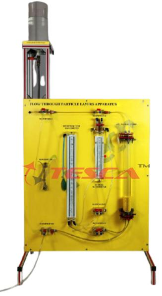
determine the pressure loss via the fixed bed or fluidized bed, two manometers with different measuring ranges are provided. The desired manometer is selected by way of valves.
