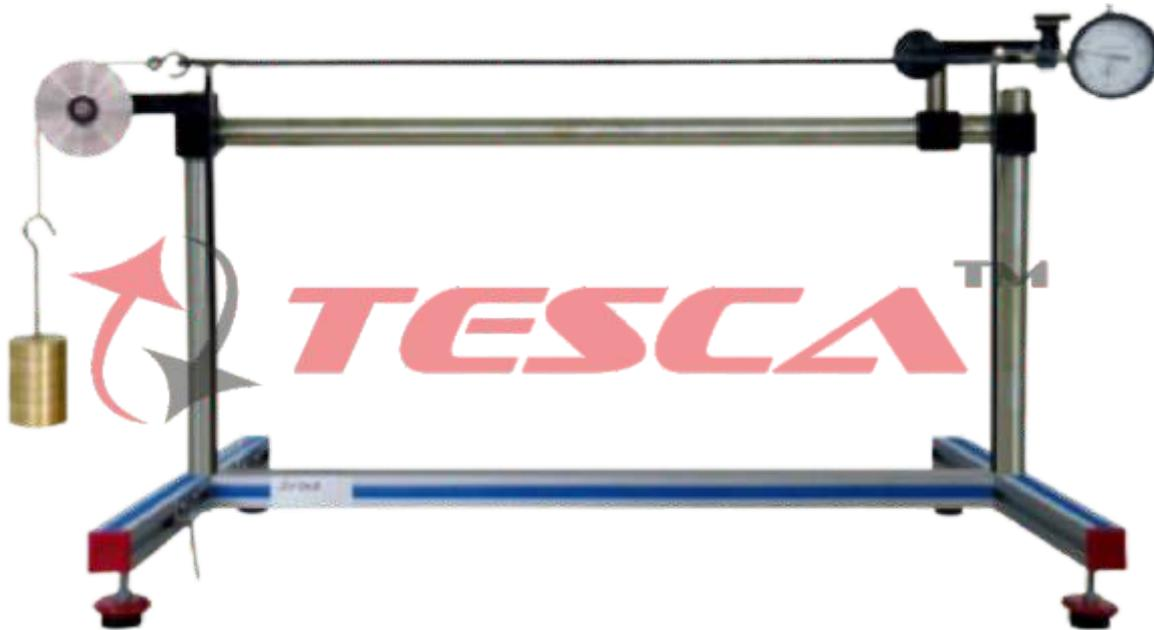
Tesca Portal Frame Unit has been designed to determine the deflection at the load point for a rectangular portal frame subjected to horizontal and vertical loads. The system is formed by a frame attached to a rigid base and loads can be applied by mass hangers and a range of masses or weights. The horizontal and vertical deflections of the frame can be measured by means of dial gauges.
