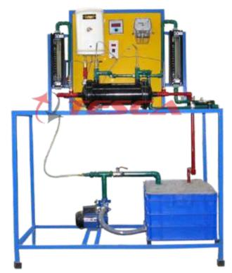
Tubular heat exchangers are often used for heating or cooling gaseous media, such as air coolers for internal combustion engines. Hot water flows in the tubes, which are surrounded by a flowing gaseous medium, e.g. cold air. The hot medium emits some of its thermal energy to the cold medium.
