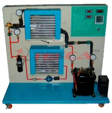
Tesca Basic Table Top Refrigeration Trainer 32400 is designed to provide students with a thorough understanding of various types of systems used in commercial and industrial applications. It permits students to understand the refrigeration cycle, including measurement of pressure, vacuum, flow rate and temperature.
