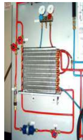
Flow Meter & Charging Gauges
