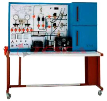
Tesca Industrial Refrigeration Trainer 32418 consists of industrial refrigeration components completely factory assembled and wired. It is designed to provide training with larger commercial and industrial refrigeration systems which require water-cooled condensers (tube-in-tube and shell-in-tube), electric and hot gas defrost systems, cooling towers, hot bypass capacity control systems, crankcase pressure regulators, crankcase heaters and pressure pumps.
