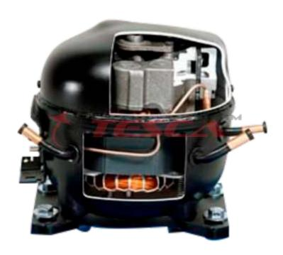
The expertly-sectioned example of a common fractional-horsepower refrigeration compressor, facilitates and supports practical training in compressor design, operating principles, and maintenance.
