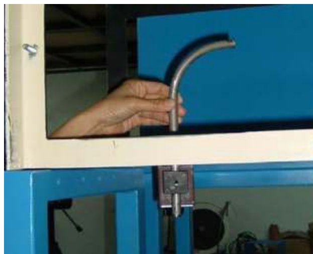
1 Place the smoke nozzle pipe into the test section
