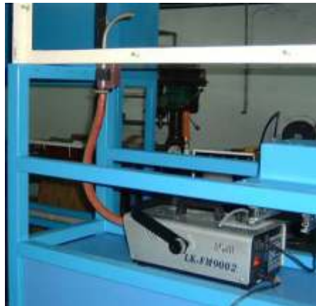
2 Align nozzle pipe into pipe holder magnetic block, and switch on the magnetic
