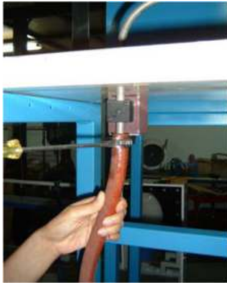
2 Align nozzle pipe into pipe holder magnetic block, and switch on the magnetic
