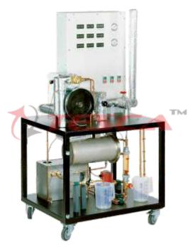
Tesca Steam Motor & Energy Conversion Test Kit 32458 is a mobile laboratory-scale steam plant for experiments in thermodynamic principles.
