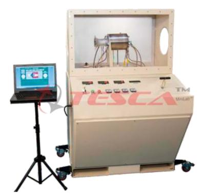
Tesca Turbo-Jet Trainer with Reheat 32468 is a fully instrumented, educational single shaft gas turbine with reheat. Powered by kerosene, the experimental abilities of this high-quality apparatus enable comprehensive practical investigations into the principles, and performance of single-shaft gas turbines with reheat.
