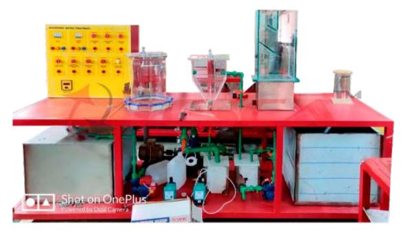
Tesca Aerobic Water Treatment Pilot Plant 32485 is an activated sludge pilot plant consists of an oxidation reactor and of a settler according to the traditional diagram of single-stage sewage treatment process.
