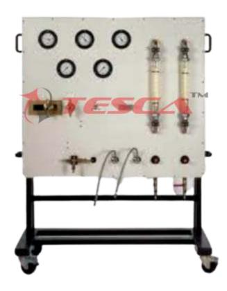
Sanitation Fittings Trainer Order Code: 32494 can be connected and investigated in respect of their function and operation on this trainer. The trainer provides several methods of connection so additional products from different manufacturers can be used. Some connectors are flexible and will adapt to different sized fittings.
