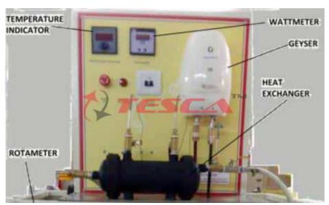
The flow rate in the hot water circuit is adjusted by means of valves. The temperatures of the water in the flow pipe, in the return pipe and in the water tank are displayed. The flow rate is displayed by means of a rotameter. Two sight glasses indicate the lowest and the highest water level.
