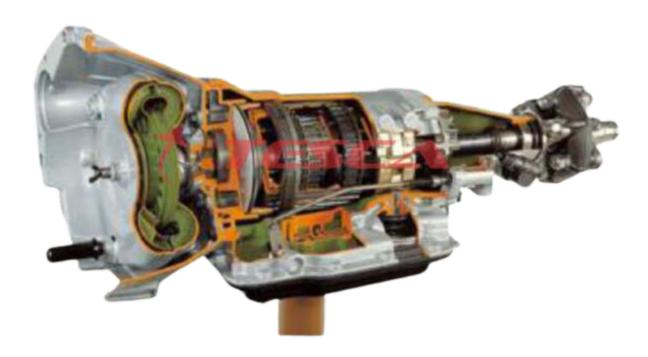
Transmission System Order Code: 32566 carefully sectioned, complete with hydraulic converter and epicyclical gear change with 3 forward speeds + reverse. The torque converter, epicyclical braking system, multiple-plate clutches and control valves are clearly shown. The transmission unit operated by a crank handle applied on the converter.
