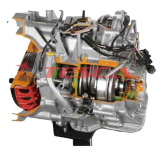
Special Gearbox that can change continuously through an infinite number of effective gear ratios between maximum and minimum values. There are two V belt pulleys that are split perpendicular to their axes of rotation, with a V belt running into them.
