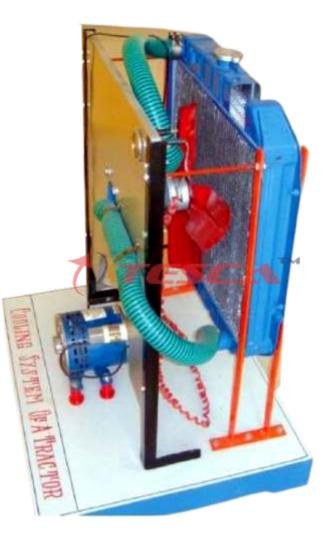
Cooling System Order Code : 32625 consists of a working of a cooling system of a car is shown with the help of actual parts assembled on a metal stand. All the necessary parts of a cooling system of a car are shown in actual working form. This model helps the student to understand the working of the cooling system of a car very easily. It is specially made dissectible for demonstration purposes.
