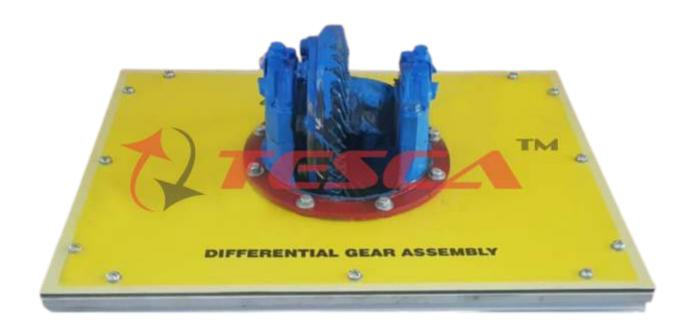
Differential Gear Assembly Order Code : 32633 is an actual Cut Section. The working of differential gear is shown with the help of actual parts assembled on square iron pipe frame. All the necessary parts of differential gear are shown in actual working form. This model helps the student to understand the working of the differential gear very easily. It is specially made dissectible for demonstration purposes.
