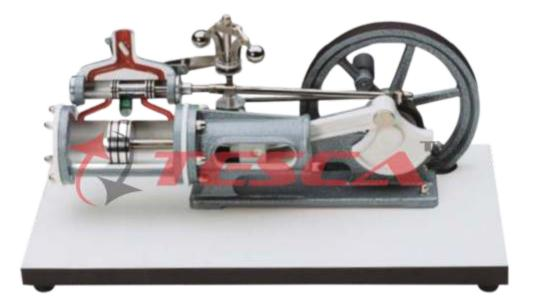
Instructive model of a modern horizontal steam engine with piston valve control. The model can be put in motion by turning the flywheel, thus showing the manner of operation of the engine and of the built-on centrifugal governor.
