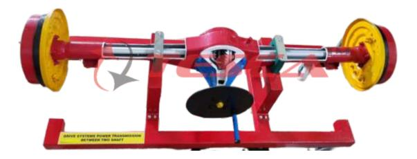
Rear Wheels with Axle with Differential Gears Assembly Order Code : 32639 Rigid rear axle complete with differential unit, axle shafts and rear drum brakes, carefully sectioned to show the operation of the differential unit where planetary gears, the ring gear and the pinion are clearly displayed. A brake drum and a cylinder are sectioned too.
