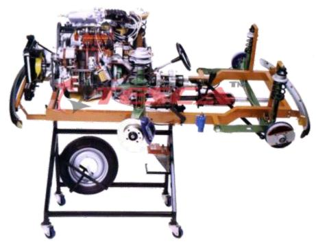
Chassis Front - Wheel Drive Diesel Engine Indirect Injection Rotating Distributor Overhead Camshaft with working Lighting System and Fully Operating Brakes
