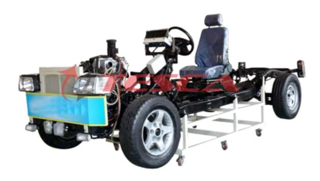
Structure Educational System of Automatic Petrol Car with Electrical Fault Simulator Order Code: 32675 demonstrates the inter-relationship between components of an actual car. The training model is built with the original automotive parts, fitted on a frame specially built by us. It is equipped with petrol engine- 4 cylinders in line with water cooling.
