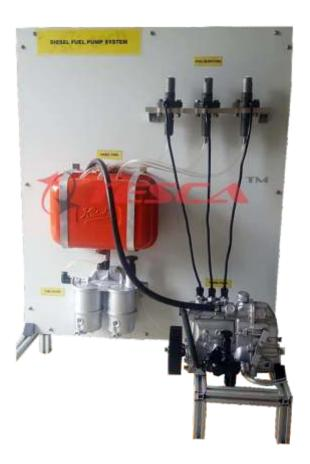
Automotive Diesel Fuel Injection System Order Code: 32681 is motorized operating type and includes diesel fuel supply system.
