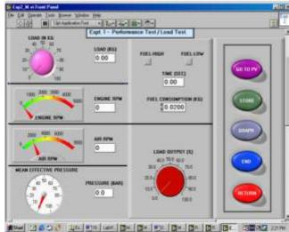
efficiency of internal combustion engine including heat balance sheet. The Engine & Dynamometer is mounted on base structure. Sci-tech Engineers have design the system in such faction that easily operate; demonstrated & requisite experimentation can be performed. System has facility of measuring Engine brake load, speed, consumption of air, consumption of fuel, temperature at different locations, mass flow of water.
