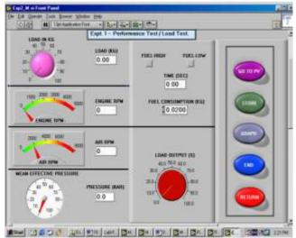
heat balance sheet. The Engine & Dynamometer is mounted on base structure. Sci-tech Engineers have design the system in such faction that easily operate; demonstrated & requisite experimentation can be performed. System has facility of measuring Engine brake load, speed, consumption of air, consumption of fuel, temperature at different locations, mass flow of water.
