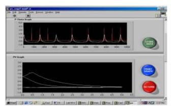
automatic calculating all efficiency & heat balance sheet of internal combustion engine. The online graphical representation of important parameter is displayed on screen to see effect of change in load or speed. Final result & graph are in built available in software. System has facility of measuring Engine brake load, speed, consumption of air, consumption of fuel, temperature at different locations, mass flow of water.
