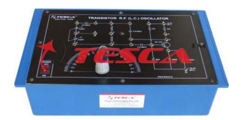
Experiment Training Board has been designed specifically for the study of Transistor RF Oscillators such as (i) Hartley's (ii) Colpitt's and (iii) Clapp's Oscillators using L-C.
