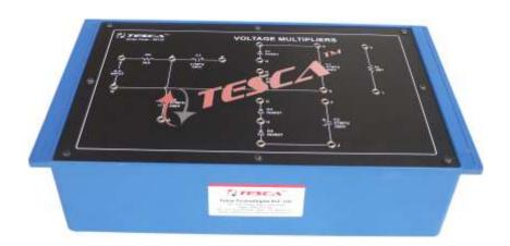
Experimental Training Board has been designed specifically to study the Voltage Multipliers such as Voltage Doubler, Voltage Tripler and Voltage Quadrupler and to determine their regulation characteristics.
