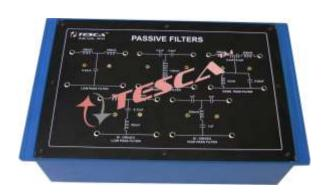
Experimental Training Board has been designed specifically to study the various types of Passive Filters and to determine the different constants as well as cut-off frequency of that particular passive filter.
