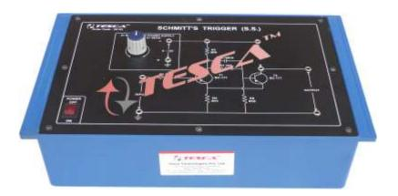
Experimental Training Board has been designed specifically for the study of Schmitt's transistor binary circuit. Study of this circuit is useful for digital electronics.
