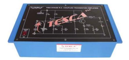
Experimental Training Board has been designed specifically for the study of Two Stage R-C Coupled Transistor Amplifier.
