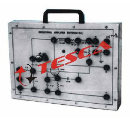
Experimental Training Board has been designed specifically for the study of Operational Amplifier.
