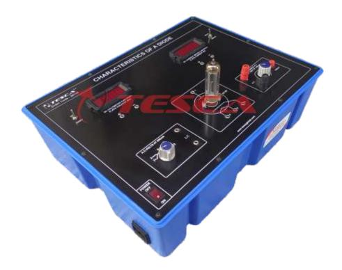
36149 Experimental Training Board has been designed specifically for the study of the Characteristics of Vacuum Diode. The board is absolutely self contained and requires no other apparatus.
