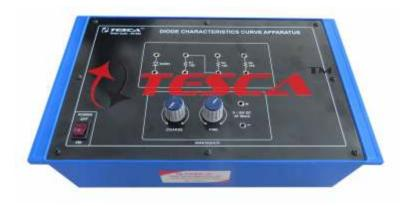
Experimental Training Board has been designed specifically for plotting Characteristics of Ge & Si Semiconductor Diodes. The board is absolutely self contained and requires no other apparatus.
