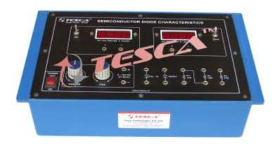
Experimental Training Board has been designed specifically for plotting Characteristics of Ge & Si Semiconductor Diodes. The board is absolutely self-contained and requires no other apparatus.
