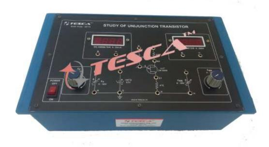
Experimental Training Board has been designed specifically to study different properties of Unijunction Transistor.
