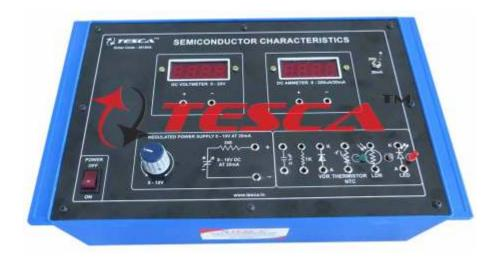
Experimental Training Board has been designed specifically to study the Characteristics of a large family of Semiconductor Devices.
