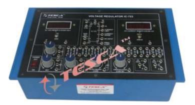
Experimental Training Board has been designed specifically to study Voltage Regulator IC 723. This Training Board gives a thorough understanding of the basic parameters of IC 723, their measurement and also covers useful applications of this regulator IC. The board is absolutely self contained and requires no other apparatus.
